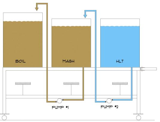
To sparge turn pumps off and move the recirculating hose from the mash kettle to the boil kettle and the HLT to the mash, then turn the pumps back on. Adjust flow rate on the pumps to the desired flow until sparging is complete.
